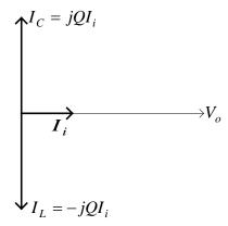
As it can be seen at resonance depending on the Q factor,  $I_L$  and  $I_C$  can be many times the supply current (current amplification).
