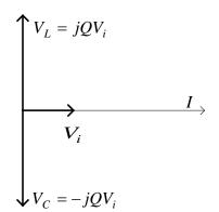
As it can be seen at resonance depending on the Q factor,  $V_L$  and  $V_C$  can be many times the supply voltage (voltage amplification).
