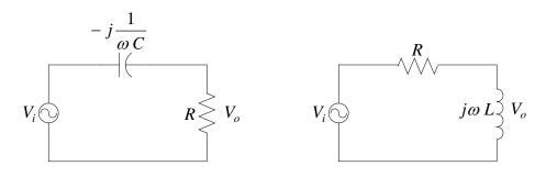
$$\frac{V_0}{V_i} = \frac{\omega RC}{\omega RC - j1}$$
